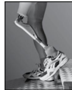
angle of the knee joint and the loading of the foot and ankle, at a rate of 50 times per second; its onboard microprocessors adapt and
