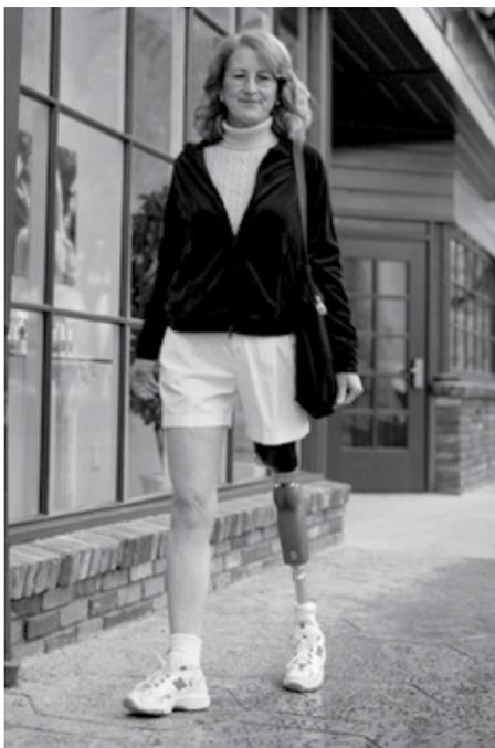
The **OSSUR RHEO KNEE®** promises its wearer less fatigue and more confidence, since it has been billed as the first artificially intelligent knee system that has sensors that relay the wearer's knee position and foot and ankle load at 1,000 times per second. This helps determine the wearer's gait and provides the proper amount of swing and stance resistance, resulting in a continually improved and optimized performance. The Ossur Rheo Knee is operational with
